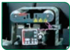
Web guide sensor - edge sensor, Line camera (Option) Correct the media path to the right spot
